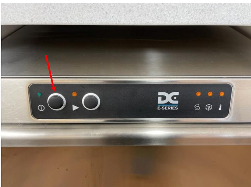
The water will immediately start draining from the machine, falling silent when draining is complete.
