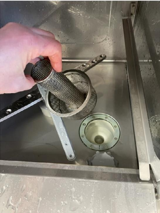
11. Replace the strainer and the drain plug, ensuring the drain plug is fully inserted (slight rotation may be needed).
