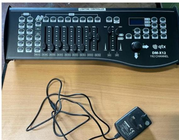
Plug the power lead into the wall and into the back of the Lighting Board.
