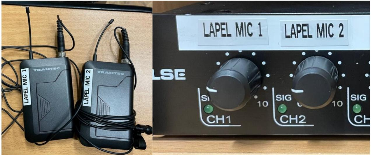
There are 2 clip-on lapel microphones in the basket on the inside of the door of the Comms Cabinet. They are labelled 1 and 2, which corresponds to the numbered dials on the amplifier in the Comms Cabinet.
