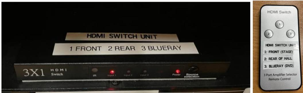
As previously described, this unit, located in the uppermost position in the 'stack', should be set to position 1 for all use of laptops and I pads on the Stage.
