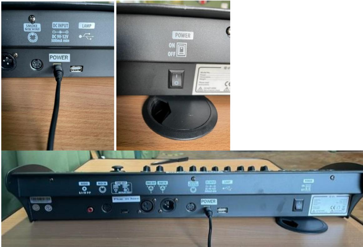
Locate the lead indicated in the photo below (red arrow) and plug the loose end of it into the back of the Lighting Control Board. It will only fit in one socket.
